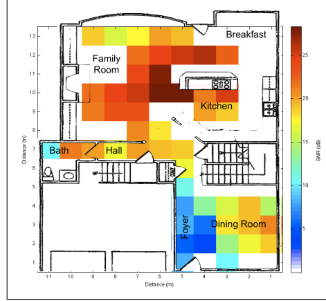
Fig. 7. A heat-map of the test home first floor indicating the Signal-to-Noise Ratio (SNR) for a 27.12 MHz wireless transmitter at each indicated location as received by a fixed powerline coupled receiver in the basement. The transmitter utilized an output power of -25 dBm ( 3.2 \mu\text{W} ) and a custom-built 27 MHz loop antenna.
